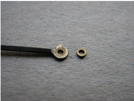
Bush in rod ready for soldering.
